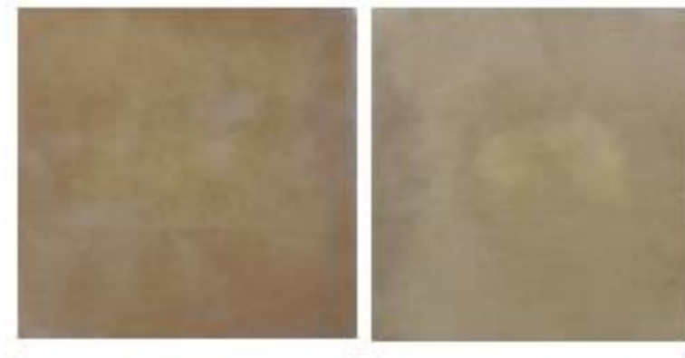
Image 3: Inconclusive result (left) obtained from inverting and pressing of moist AmylasePaper on textile stained with saliva, as opposed to a positive result (right) obtained from directly pressing of the textile stain onto AmylasePaper.
